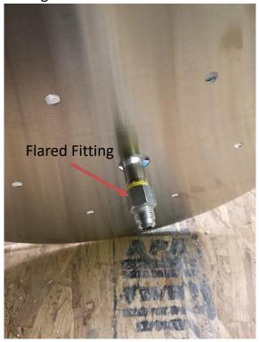
Fasten the connector line to the flared fitting. Make sure all connections are sealed and tight. Do not use Teflon ® tape or pipe sealant on any flare ends because you will not obtain a leak-free seal. Keep flare end of fitting free of grease, oil and thread sealant.
